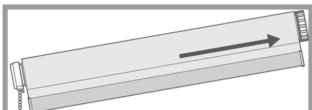
Lift the control end of the blind until level and release pressure, the blind will hold itself in place.
