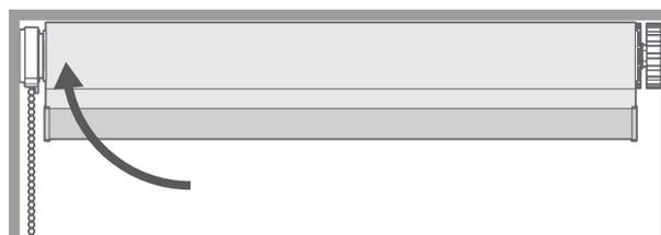
Make adjustments to the position of the blind so that it is straight and level, before locking it in place.
