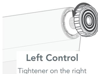
Once the blind is secured in place, turn the end cap until it locks against the tightening wheel. This will lock the tightening wheel in place.
