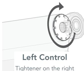
Hold the blind securely in place and turn the tightening wheel to tighten the blind in place.
