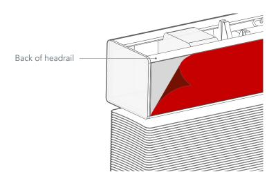
On the back of the headrail is an adhesive strip. Peel the cover from the strip, on the headrail only for now.
