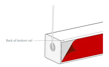
Peel the adhesive cover from the strip on the bottom rail.
