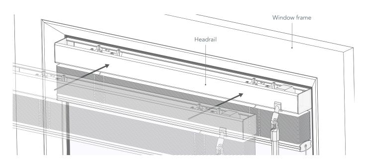
Carefully line up the headrail with the top of the visible glass. Make sure that the top of the rail is flush with the edge of the rubber, if the seal is visible, or the edge of the frame if it is not. Press the adhesive-backing to the glass and hold until it feels secure.
