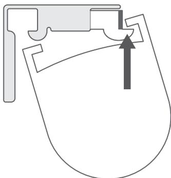
Situate the front lip of the headrail into the front of the bracket.
