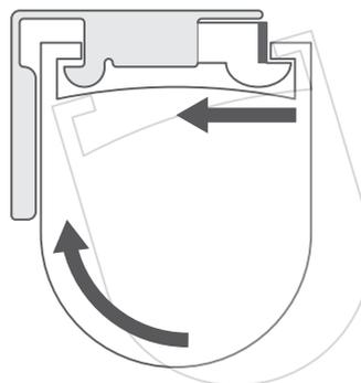
Push the back of the headrail upwards to lock it into the back of the bracket.
