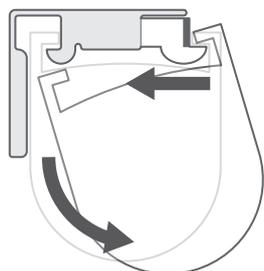
To release the blind from the brackets at any point after installing, push firmly against the blind's headrail to disengage it from the front of the bracket. At the same time, twist the back of the headrail downwards to release it from the back.
