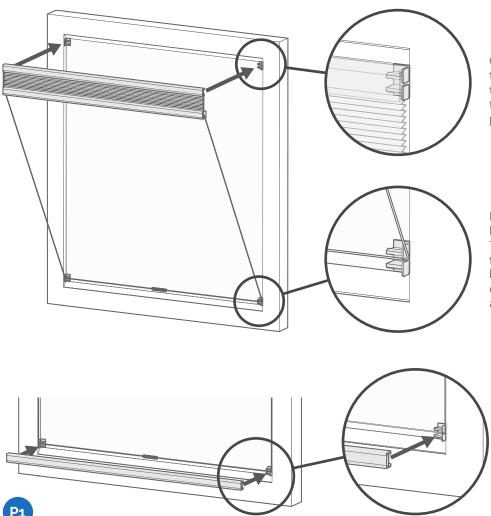
Clip the headrail onto the brackets at the top of the window by aligning the rail with the brackets and pushing the rail back towards the glass until you hear it click into place.
