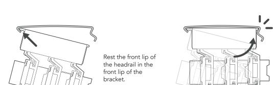
Then twist the back of the headrail upwards until it snaps into place in the rear hook of the bracket.
