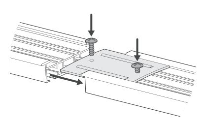
If your width is greater than 2600mm, you will be provided with 2 tracks and a joining plate to connect them together.
