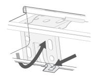
To remove the blind from the brackets, insert a flat head screwdriver into the tab protruding from the bottom of the rail, then gently pry it back while tilting the back of the rail downwards. Repeat this carefully for each bracket to release the rail.
